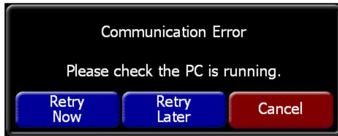
*(This means the till cannot contact the Pos Integration service on the PC.)*
