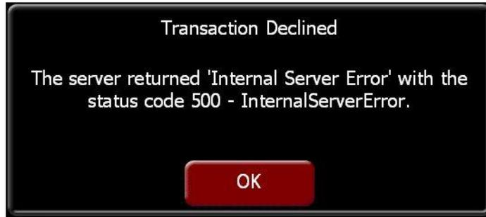
If the internet connection is being routed through a proxy and the login credentials aren't correct then the user will see this dialog at the POS:
