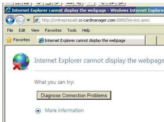
If this returns ok and ZonalCLMService is running then means access between till and service could be blocked on a network/port level – IT issue
